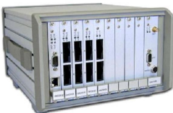
**Figura 3.3: Vista Frontal del chasis GWMP8000.<sup>15</sup>**
