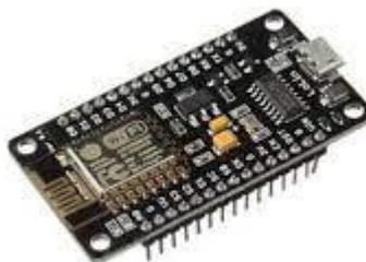
Figura 2. Placa ESP8266NodeMCU
