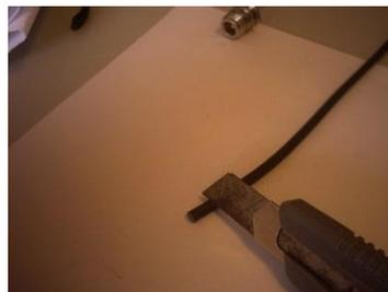
**Figura 58.** Corte cable coaxial RG58
