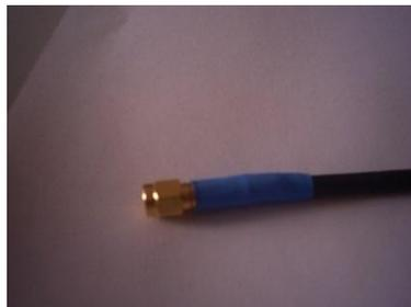
**Figura 66.** Ponchado final SMA y coaxial RG58
