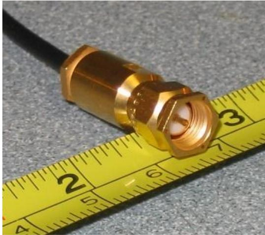
**Figura 13.** Conector SMA.
