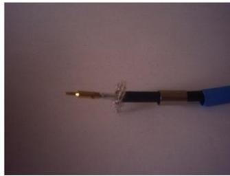
**Figura 60.** Conector SMA al cable RG58
