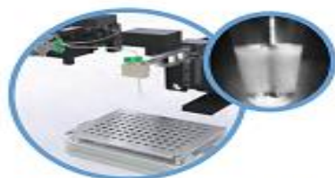
Fig. 1.6. QX200 Droplet Reader autosampler.
