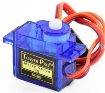
Figura 15: Servomotor Tower Pro SG90 [20].
