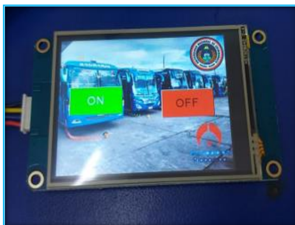
Figura 2.4: Pantalla Nextion NX3224T028 2.8 inch
